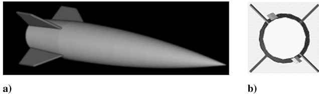
Fig. 1 Three-dimensional rendering of models for blind simulations: a) baseline configuration, and b) aft view of projectile with trapezoidal control pins.
